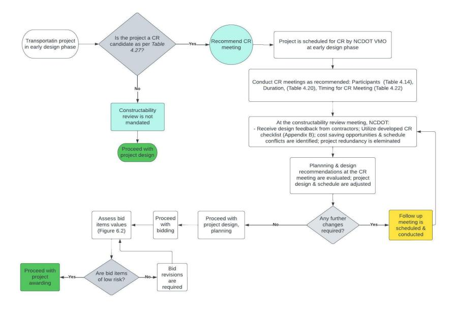
Figure 7.2: Recommended constructability review process for NCDOT
